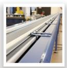
Painted Steel Mat Top Conveyor: features durable carbon steel construction for bulk conveying in industries that do not require wash down. This mat top conveyor is extremely customizable.
