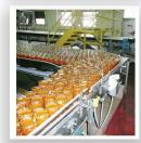
Simpli-Mat® Aluminum Conveyor: provides light-duty bulk handling, utilizing a modular aluminum conveyor design. This reconfigurable conveyor system is simple to integrate and can be easily upgraded.
